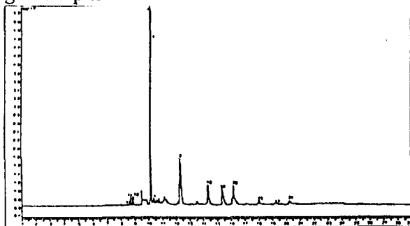
A normal sample with No.4, 2, and 26 as the dominant glucosinolate as well as the three sulphinyl glucosinolates No.10,11, and 12.
