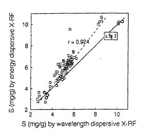
To solve this problem and in order to investigate the suitability of energy dispersive X-RF for total glucosinolate analysis all samples with sulphur concentrations above 0.7% has been excluded and after that the total sulphur concentrations obtained from the energy dispersive X-RF (X) were fitted to the values of the wavelength dispersive system (Y) by a linear transformation: Y = 0.686\*X + 1.055.
