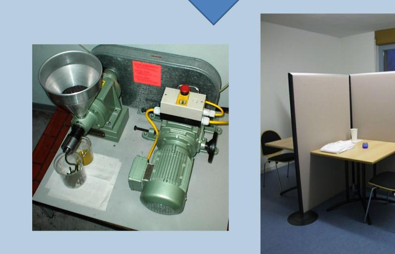
**Pressing** of rapeseed by a screw press and sensory evaluation of the resulting oils by a trained panel.
