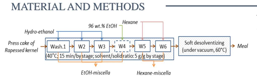
The press cake was first extracted by a succession of washing-filtration steps by solvents in an agitated Nutsche filter (POPE Scientific Inc., USA). Three extraction sequences were compared:
