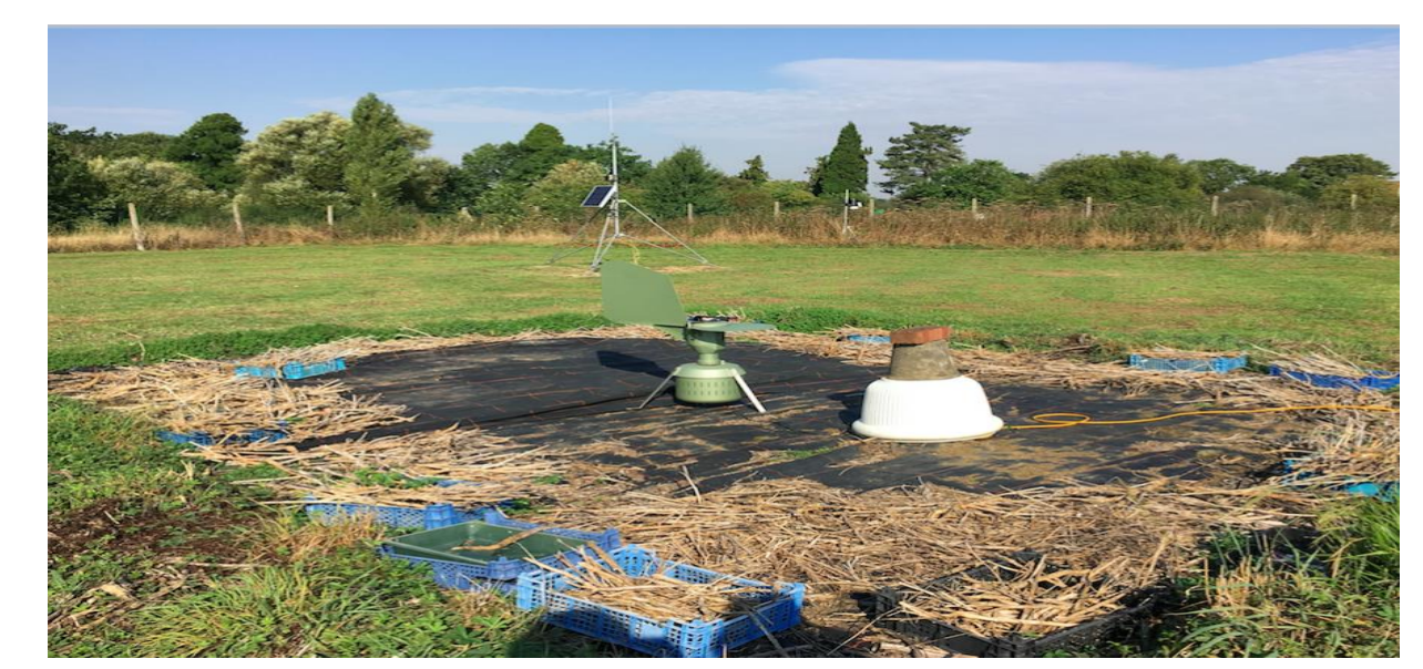
Fig 2: Burkard air sampler set up at Bayfordbury in Hertfordshire
