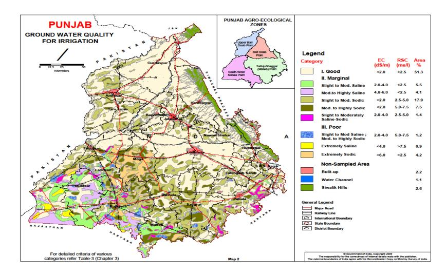
Out of 42 % poor quality ground waters, 25 % are saline, 69 % are sodic and 6 % are saline-sodic in nature.
