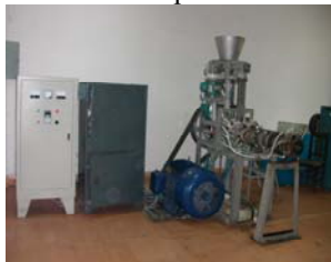
Fig 1 Dry-single-screw extruder for high-oil-content material developed in the experiment
