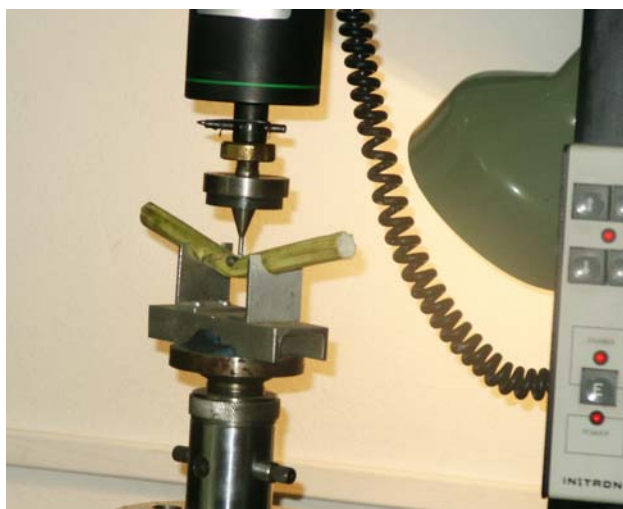
Fot. 1. Stem bending in the INSTRON device.
