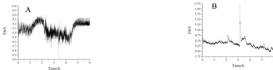
Fig. 3. The oxygen bursts variation within the natural oilseed rape lamina induced by salicylic acid detected by using micro-sensor based on Pt/Pt/POPD electrode. Constant potential: -0.1 V. A: susceptible oilseed rape genotype, 84039; B: Glucose oxidase (GO)-transgenic oilseed rape, GO16
